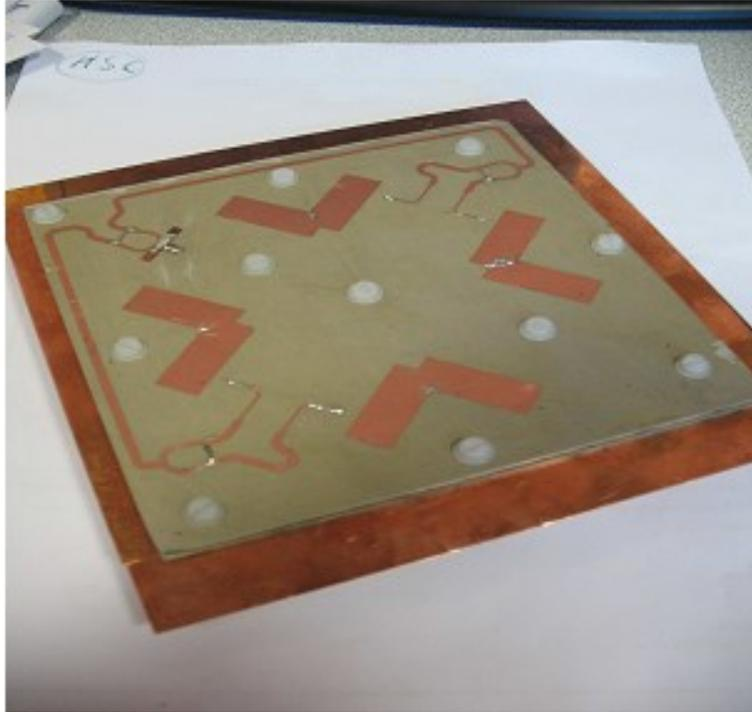
Figure 5.22: Realized patch array antenna on Rogers 6006 substrate (tm)
