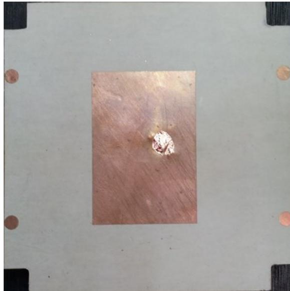
Figure 5.8: Realized patch antenna on Rogers 6002 substrate (tm)
