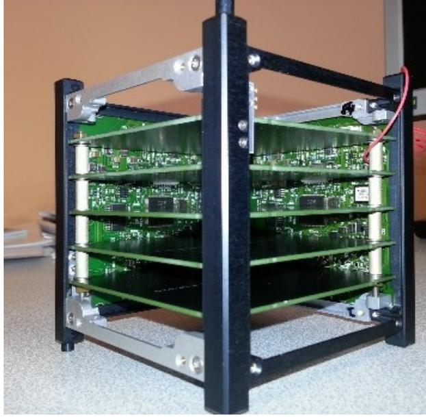
Figure 2.9: ISIS 1-Unit CubeSat structure
