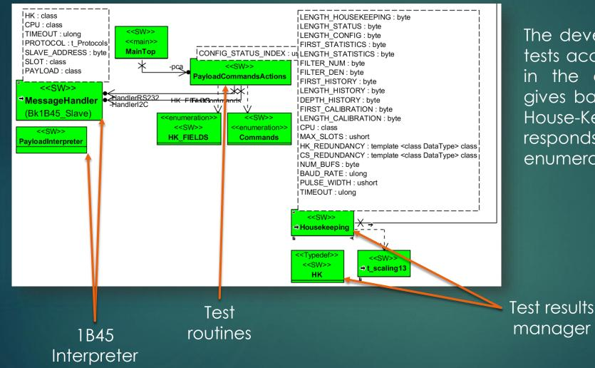
The developed software class starts the tests according to the commands listed in the enumeration Commands and gives back the results using the AraMIS House-Keeping management who responds to the requests listed in the enumeration HK\_FIELDS
