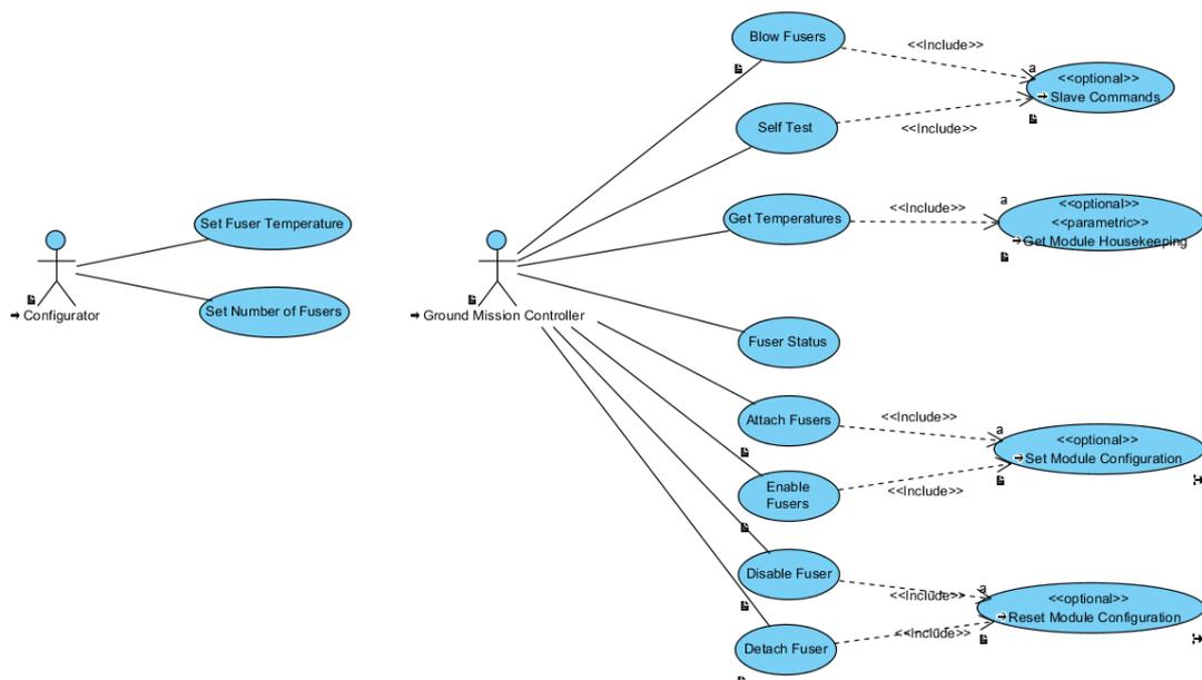
Figure 98: Use Case Diagram of the Outer Plate.
