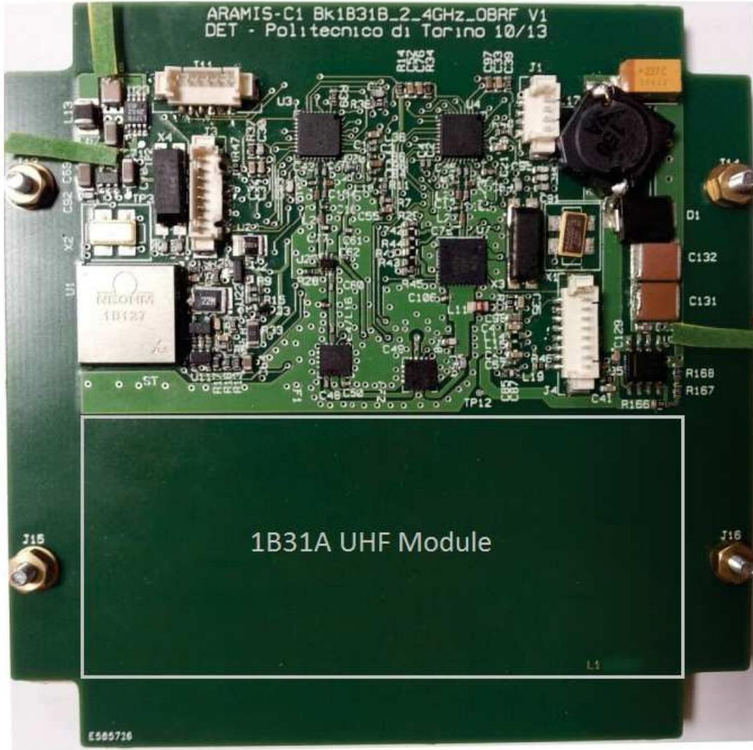
Figure 7.1. The implementation of half tile with the 1B31B OBRF and the available space for the UHF module
