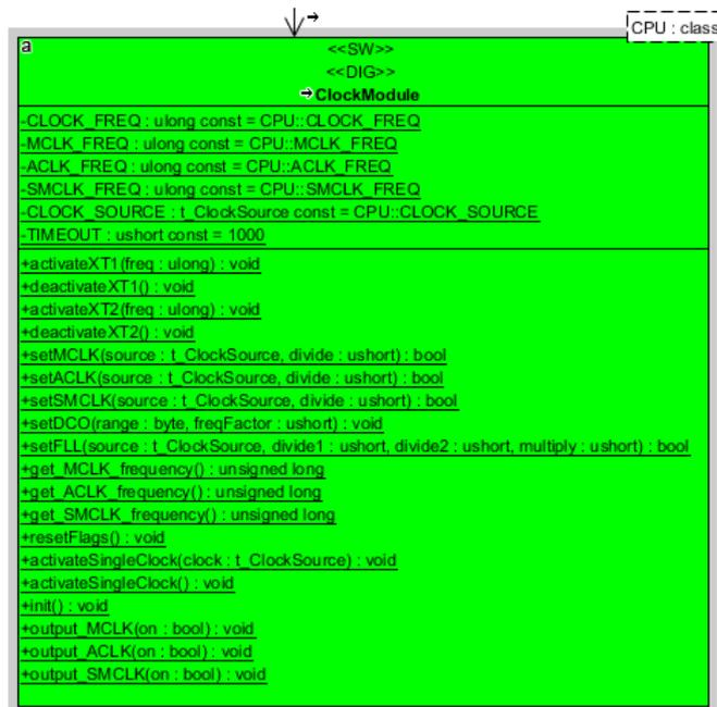
Figure 2.6: Clock Module Class diagram
