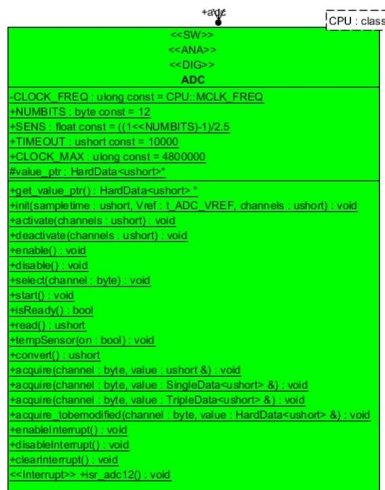
Figure 5.2: ADC Module Class diagrams
