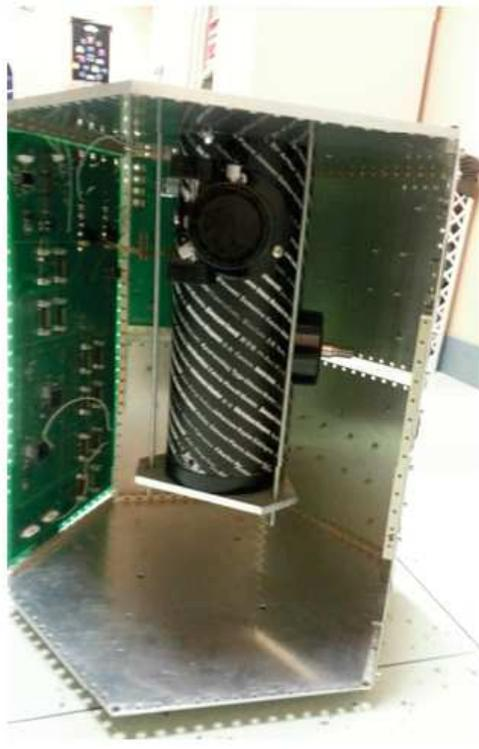
Figure 6.8. Honeycomb tiles assembled in hexagonal shaped spacecraft with optical telescope payload (mock-up)
