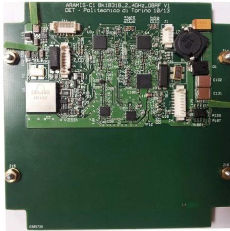
Figure 5.2. Cube Telecommunication Tile
