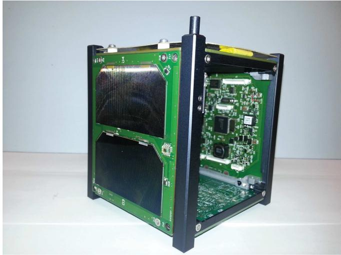
Figure 5.4. AraMiS Satellite on Demand configuration fabricated using 1B8 CubePMT and 1B9 CubeTCT
