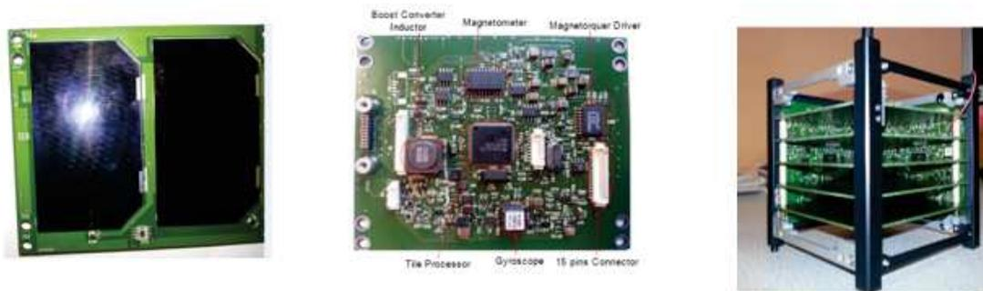
Figure 2.3. Photograph of 1U CubeSat compatible tile (a) External view (b) Internal view (c) arranged in 1U configuration
