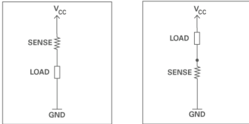
Fig. 3 - 6 : High Side Versus Low Side Current Measurement
